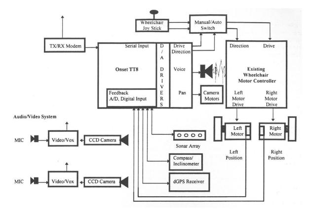
Figure 1. Onboard System Diagram.
