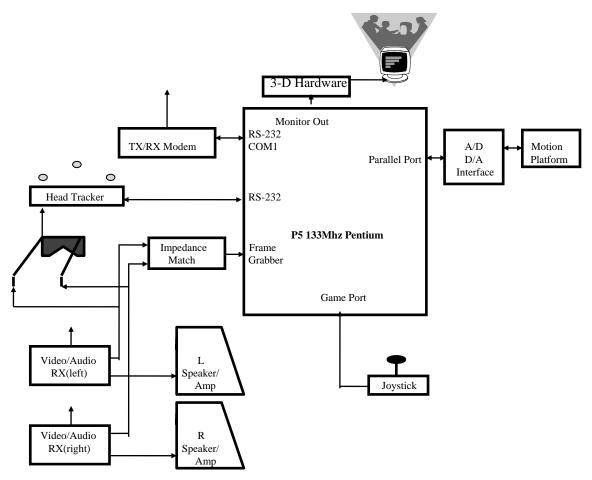
Figure 2. Remote Control System Diagram.
