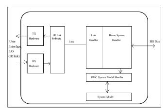
Figure 1. Schematic of the User Interface Feature Controller
