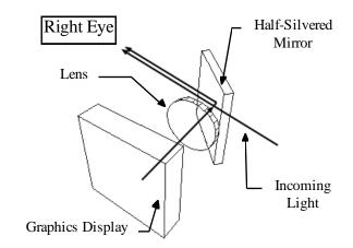
Figure 3. Basic Optical Configuration (Right Hand Side)
