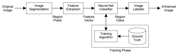
Figure 4. Architecture of Image Enhancement System
