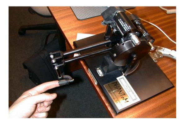
Figure 1. The PHANToM 1.0 with thimble interaction device
