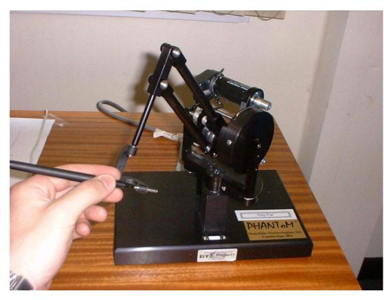
Figure 2. The PHANToM 1.0 with stylus interaction device
