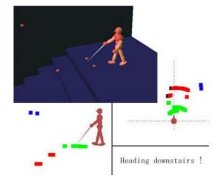
Figure 7. The simulation result of surroundings presumption for a downstairs.
