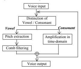
Figure 2. Flow diagram of filtering
