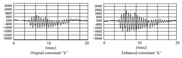
Figure 6. Waveforms of consonant "k" before and after the filtering
