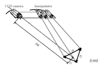
Figure 3. The design of active-stereo range sensor
