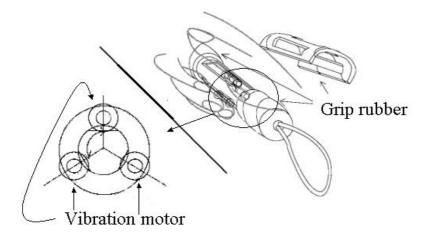
Figure 4. The design of tactile display
