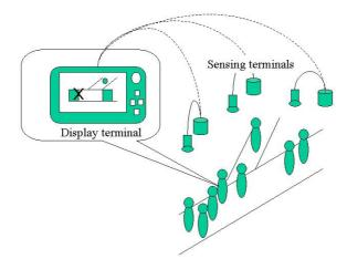
Figure 6. The conceptual design of traffic flow sensing system
