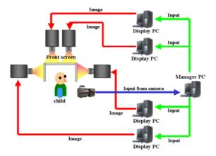
Figure 2. Block diagram of proposed system.
