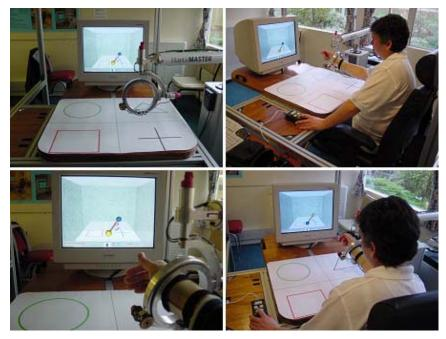
**Figure 3.** Subject using the Gentle/s prototype system with one of the available virtual rooms. The virtual environment replicates the user's viewpoint in the real world where the mat with shapes is used to help perception of movement and space.
