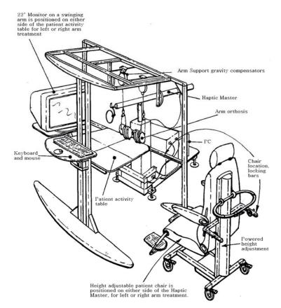
**Figure 1.** The Gentle/s prototype system, showing the overall frame, an elbow orthosis suspended from the overhead frame, the HapticMaster with gimbals, the exercise table, computer screen and the wheelchair.
