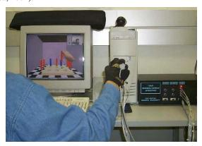
Figure 2. Rutgers Haptic Master being used to reflect grasp force during virtual chess match.
