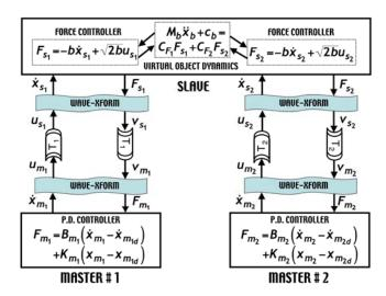
Figure 7. Wave variable control architecture.
