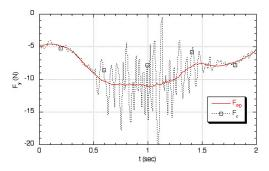
**Figure 9.** Total force command  $(F_o)$  and PD component  $(F_{PD})$  in x-direction for gain of k=5.
