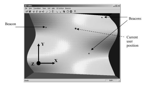
**Figure 2.** Screen snapshot of a haptic surface plot with visual representation of beacons. The user can feel the 3D surface of the table using a PHANToM haptic interface. The value of each cell is mapped to height in the z- direction.
