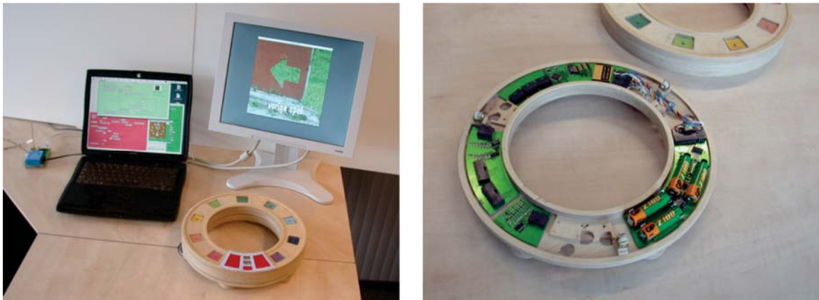
Figure 2 E-scope consists of a wooden toy, a computer with a wireless station and an optional separate monitor (left). The upper and lower ring of E-scope communicates with the computer through radio transceivers (right). All sensors, actuators and batteries are built into the layers of E-scope.
