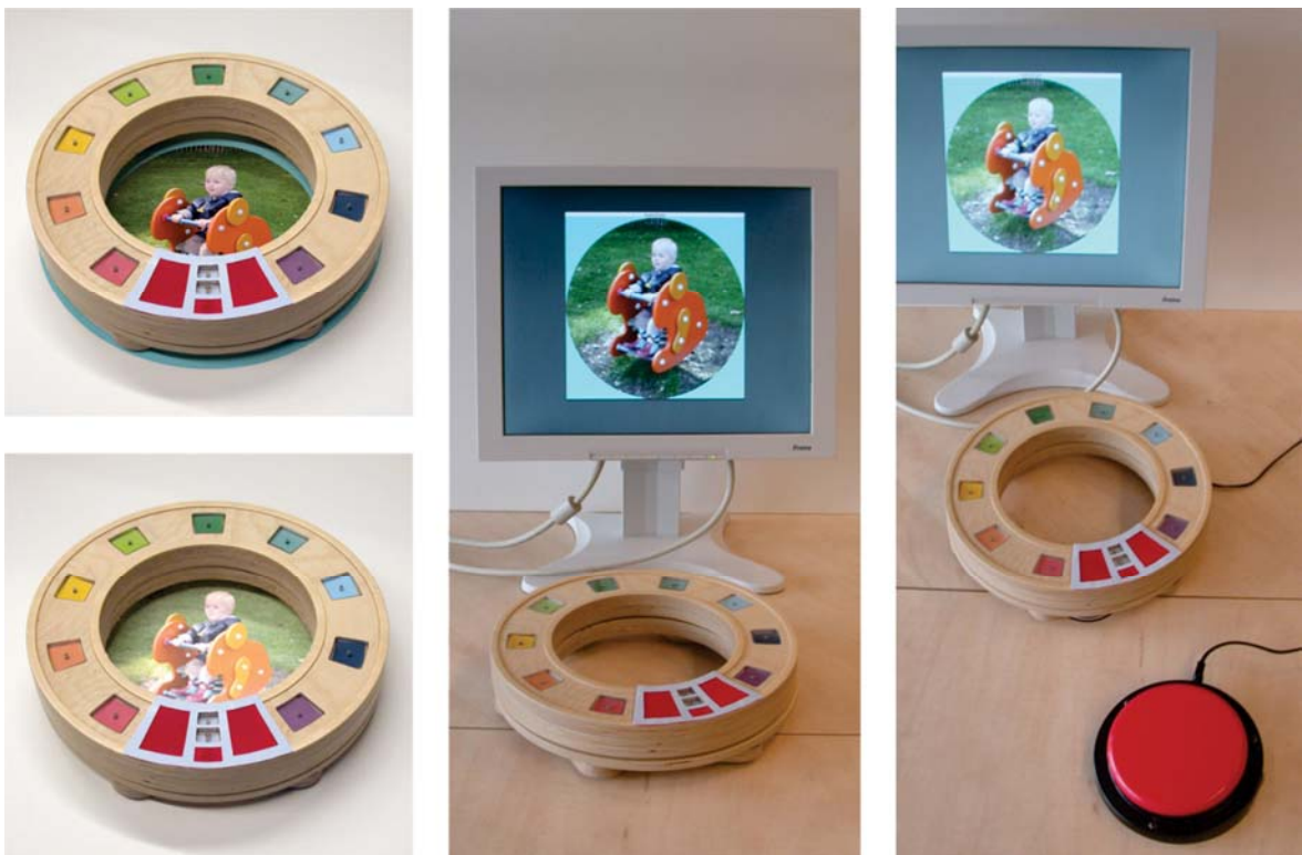
Figure 3 E-scope configurations: Using pictures (upper left); integrated LCD screen (lower left); with separate screen (centre), or with a variety of input devices making it possible for a severely motor handicapped person to operate it (right).
