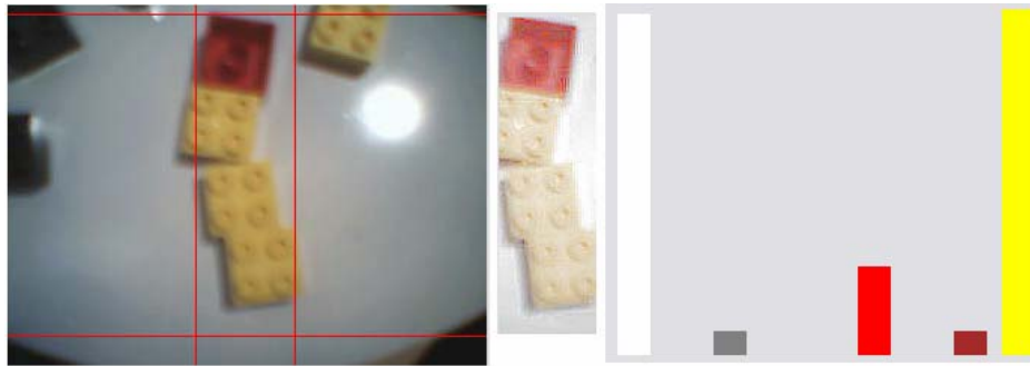
Figure 2 Screen taken before and after colour extraction
