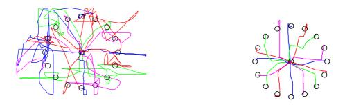
**Figure 1.** Cursor Movements of a Motion Impaired user to select a target in an undamped (left) and force-feedback damped (right) condition.
