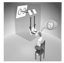
Figure 2. Concept of the desk mounted display, showing different images presented to each eye.
