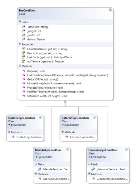
Figure 7. Hierarchical class diagram of eye conditions.
