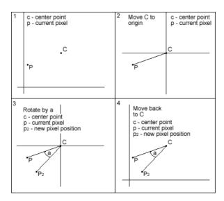
**Figure 3.** Rotation calculation - vector is found between P and C in 1 ands moved to the origin in 2; rotated by the angle (related to distance from C) in 3 and finally moved back to C in 4.
