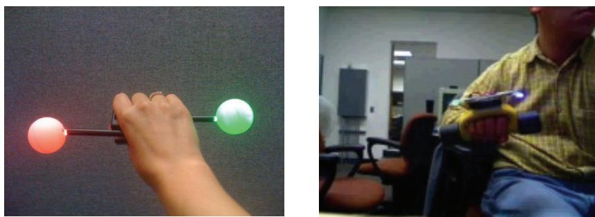
**Figure 1.** An optical tracking device that utilizes one or two low-cost webcams to track one, two or three diodes providing information of three, five, or six degrees of freedom, developed by Yeh et al. (2008).
